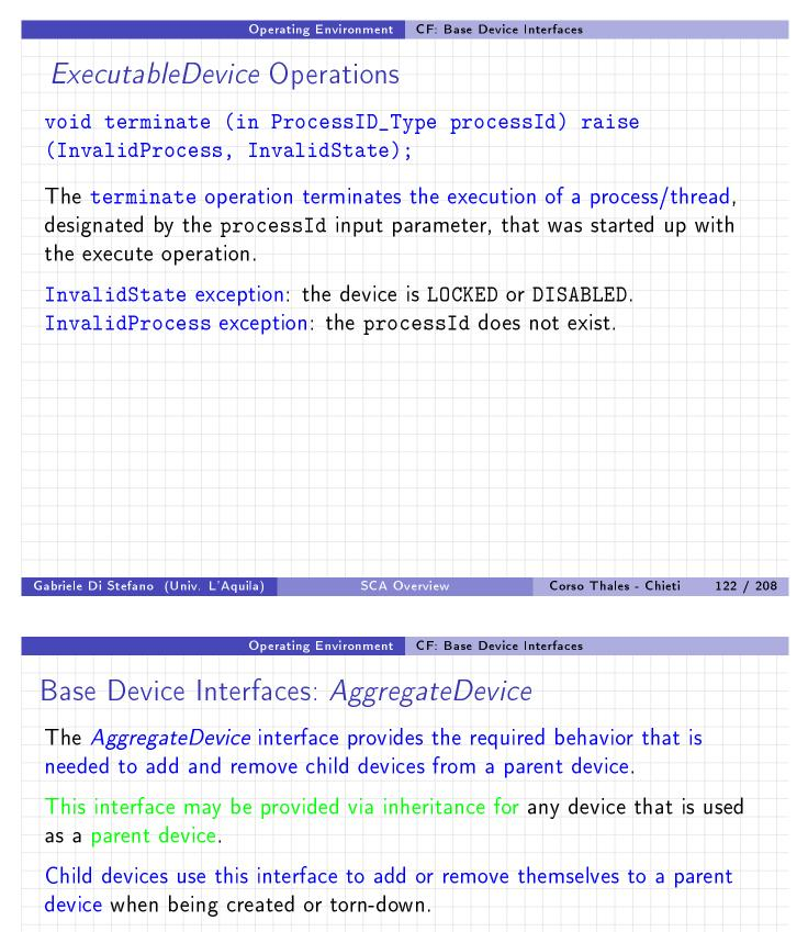
E.g., consider several FPGAs on a single card. Each FPGA would be a child device and the board that contains the FPGAs would be the parent device.
