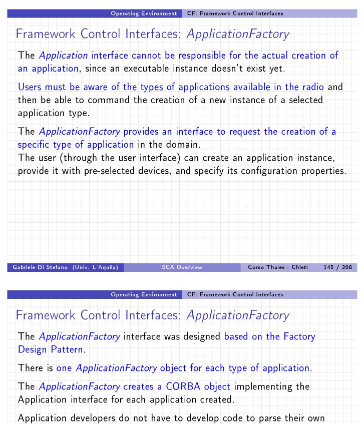
software profiles to create their application within a domain. An *ApplicationFactory* CORBA object is created for each different Software Assembly Descriptor (SAD) XML file installed in the domain.
