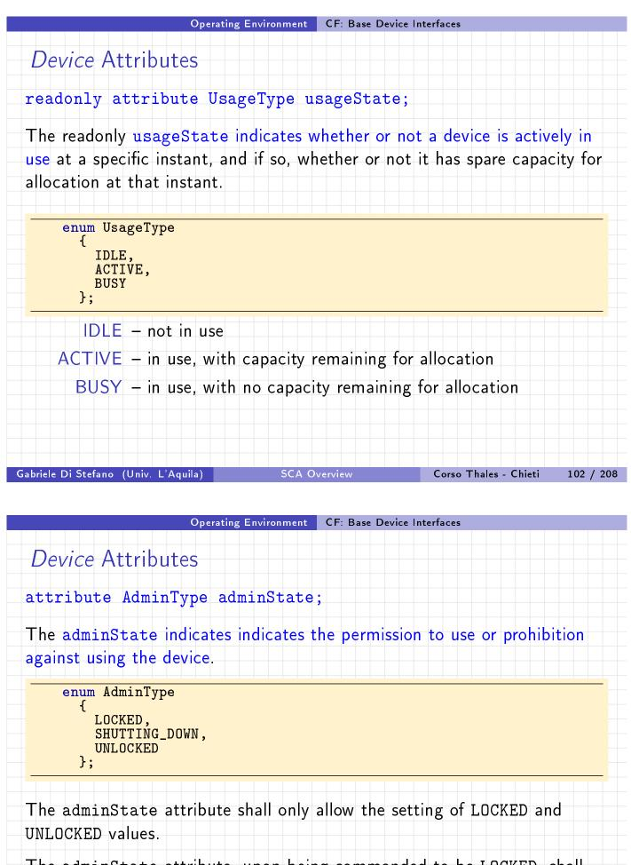
The adminState attribute, upon being commanded to be LOCKED, shall transition from UNLOCKED to SHUTTING\_DOWN and set the adminState to LOCKED for its entire aggregation of devices (if any). The adminState shall then transition to LOCKED when the device's usageState is IDLE and
